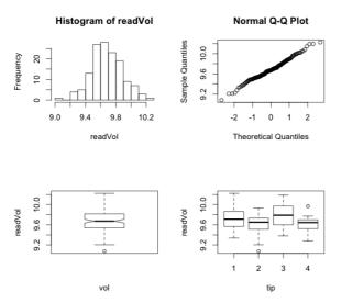
*Detecting sources of error*: The graph below shows boxplots of absorbance readouts for dye dispenses of 20ul and 50ul volume using four different, fixed tips. We see that tip 2 has much greater variability than the other tips. This allowed us to localize an important source of error and to correct it by replacing that tip.
